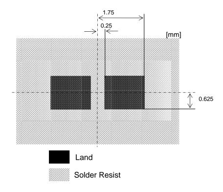
4-3. Recommended mounting pattern at antenna side for the attachment by adhesive
