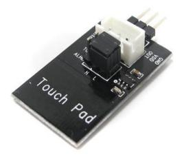
Touch button is designed for replacing traditional direct button key with diverse pad size. Low power consumption and wide operating voltage are the contact key features for many applications.
