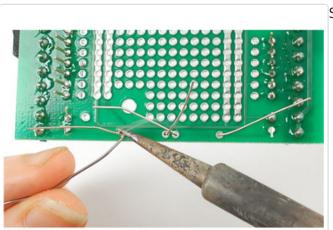
Solder and clip the two resistors.
