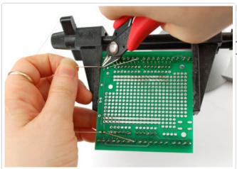
Use the diagonal cutters to clip the long LED legs. They should be cut just above the solder joint.
