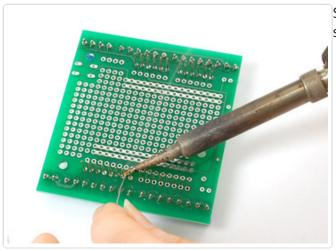
Solder all the pins of the header with plenty of solder.
