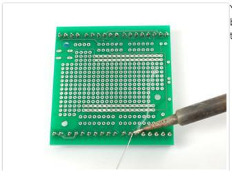
You can also just put the PCB with terminal blocks upside down on a table, which will keep the blocks in place while soldering.
