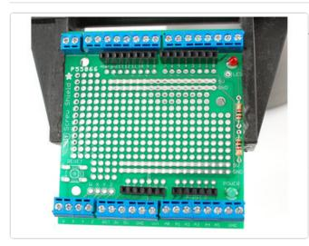
Next we will place the two 1.0Kohm resistors. These resistors are used to set the brightness of the LEDs. If you want brighter LEDs you can substitute 220 ohm resistors. If you want dimmer LEDs, you can use 4.7Kohm.
