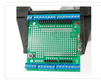
Last we will place the reset switch. This switch will let you easily reset the Arduino.
