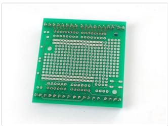
Flip over the PCB, you can lay it down on a table again, just make sure that all the headers are sticking out straight.
