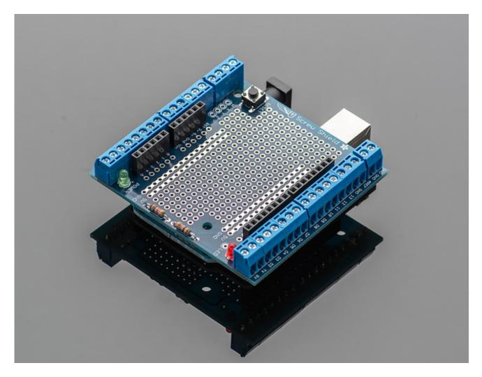
The shield even comes with stacking headers, (http://adafru.it/alH) which let you plug another shield on top! As shown here, a data logging shield is stacked onto the protoscrewshield.
