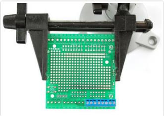
Get ready by putting the PCB in a vise. Then you can start by placing one of the 8-piece terminal blocks in the "Analog" breakout area.
