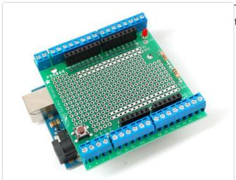
That's it! You can now insert the headers into the Arduino and start using the shield!
