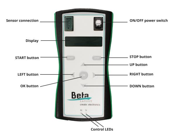
The display shows information on the current soldering process, as well as error messages.
